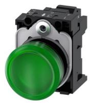
Indicator lights, 22 mm, round, plastic, green, lens, smooth, with holder, LED module, with integrated LED 24 V AC/DC, spring-type terminal, with laser labeling, lower case
