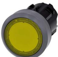
Indicator light in illuminated pushbutton design, 22 mm, round, plastic with metal front ring, yellow, with laser labeling, inscription or symbol Customer-specific selection with SIRIUS ACT configurator (CIN)
