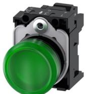
Indicator lights, 22 mm, round, plastic, green, lens, smooth, with holder, LED module, with integrated LED 110 V AC, spring-type terminal, with laser labeling, inscription or symbol Customer-specific selection with SIRIUS ACT configurator (CIN)
