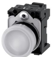
Indicator lights, 22 mm, round, metal, shiny, white, lens, smooth, with holder, LED module with integrated LED 110 V AC, spring-type terminal, with laser labeling, symbol number according to, ISO 7000 or IEC 60417
