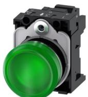
Indicator lights, 22 mm, round, Metal, shiny, green, lens, smooth, with holder, LED module with integrated LED 230 V AC, spring-type terminal, with laser labeling, upper case and lower case, always upper case at the beginning of the word
