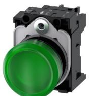
Indicator lights, 22 mm, round, plastic, green, lens, smooth, with holder, LED module, with integrated LED 230 V AC, screw terminal, with laser labeling, lower case
