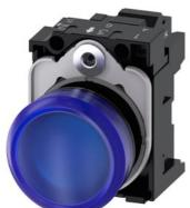
Indicator lights, 22 mm, round, plastic, blue, lens, smooth, with holder, LED module, with integrated LED 110 V AC, spring-type terminal, with laser labeling, upper case
