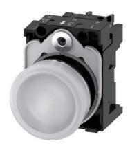
Indicator light, 22 mm, round, metal, shiny, white, lens, smooth, with holder, LED module with integrated LED 24 V AC/DC, screw terminal, with laser labeling, upper case and lower case, always upper case at beginning of line
