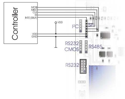
DIP-Switch setting: SPI-Interface (EA 9777-2PE)
