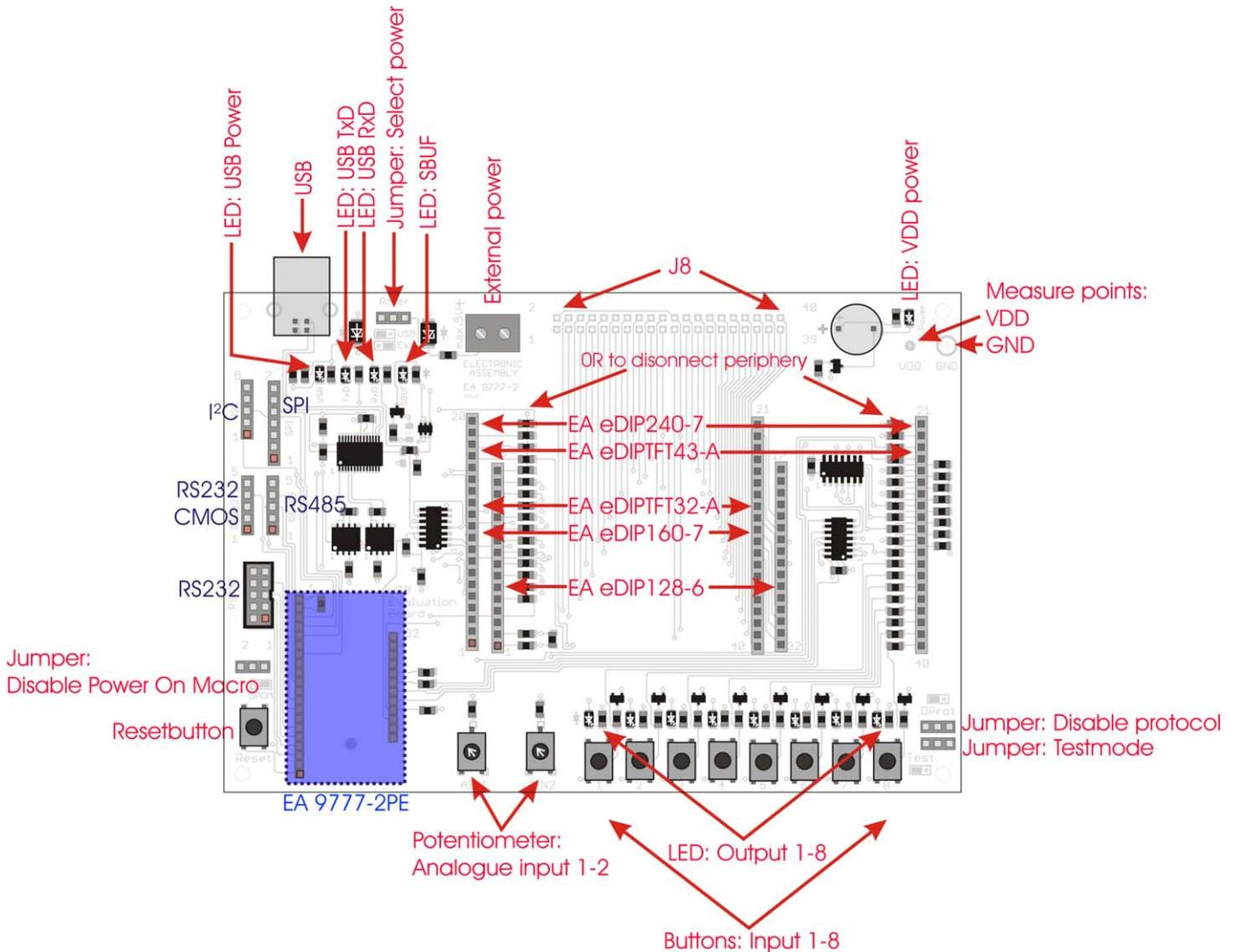
The Evaluation board provides a variety of features, starting with LEDs to indicate data-transfer, ending with potentiometers to use the analogue inputs of EA eDIPTFTs.
