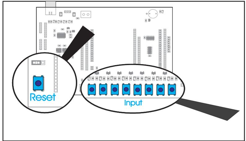
8 buttons are directly connected to the inputs of the EA eDIP. If you push a button the corresponding input is grounded. Please refer to the schematic on the last page of this datasheet.
