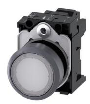
Indicator light, in illuminated pushbutton design, 22 mm, round, plastic with metal front ring, white, with holder, LED module, with integrated LED 24 V AC/DC, Spring-type terminal
