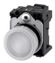
Indicator lights, 22 mm, round, metal, shiny, white, lens, smooth, with holder, LED module with integrated LED 24 V AC/DC, spring-type terminal, Z=20-unit packaging
