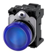
Indicator light, 22 mm, round, metal, shiny, blue, lens, smooth, with holder, LED module with integrated LED 24 V AC/DC, spring-type terminal, with laser labeling, upper case and lower case, always upper case at beginning of line
