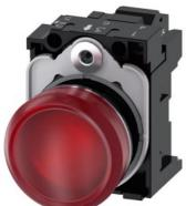
Indicator lights, 22 mm, round, metal, shiny, red, lens, smooth, with holder, LED module with integrated LED 110 V AC, spring-type terminal, with laser labeling, symbol number according to, ISO 7000 or IEC 60417
