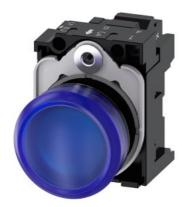
Indicator lights, 22 mm, round, plastic, blue, lens, smooth, with holder, LED module, with integrated LED 230 V AC, Spring-type terminal
