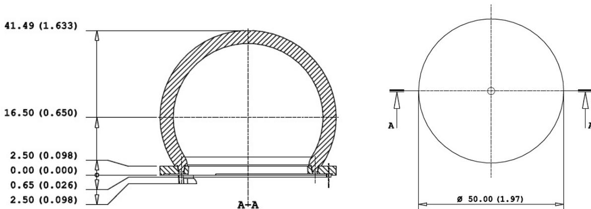
GRACE50/SEMI - Ø 50 mm - Optical Diffuser 1/2 Sphere, Twist&Lock
