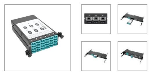
Installs in select Tripp Lite fiber enclosure panels to connect 12 LC duplex fiber cables with three 8-fiber MTP/MPO connections in high-density network applications.
