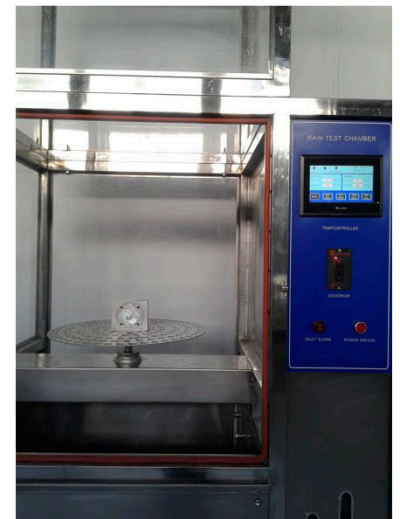
Testing under water jet
