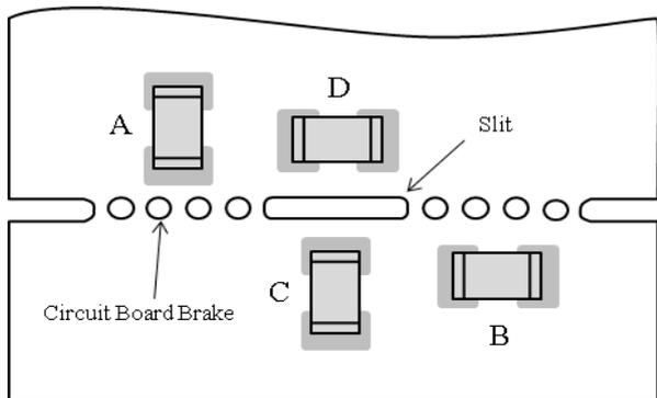
Stress strength according to the mounting position:
