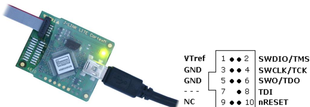
Figure 3 – SEGGER J-Link Lite Cortex-M 9-Pin JTAG with pinout (Rev 2.1+)
