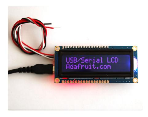
Inside the backpack is an USB-capable AT90USB162 chip that listens for commands both a mini-B USB port and a TTL serial input wire. The USB interface shows up as a COM/serial port on Windows/Mac/Linux. The backpack will automatically select data from whichever input is being used.
