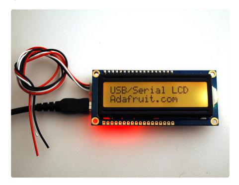
Adding a character display to your project or computer has never been easier with the new Adafruit USB or TTL serial backpack! This custom-designed PCB sits on the back of any 'standard' character LCD (16x2 or 20x4 sized) (https://adafru.it/alS) and does everything you could want: printing text, automatic scrolling, setting the backlight, adjusting contrast, making custom characters, turning on and off the cursor, etc.
