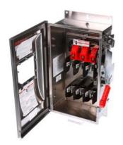
Siemens Low Voltage Circuit Protection Heavy Duty Safety Switches. Type: ENCLOSED, SAFETY SWITCH Std: CSA V. Rating: 600V A. Rating: 30 A Wattage: 3W No. Of Poles: 3P F. Rating: 60Hz Action: SINGLE THROW Material: SS Enclosure: TYPE 4X. 2-3 point mounting holes. Insulation: YES O. Cycles: 10000 O. Temperature: (-20F-120F) AMBIENT TEMPERATURE Environmental Conditions: INDUSTRIAL CORROSIVE RESISTANCE
