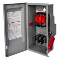
Siemens Low Voltage Circuit Protection Heavy Duty Safety Switches. Type: ENCLOSED, SAFETY SWITCH Std: CSA V. Rating: 240V A. Rating: 100A Wattage: 3W No. Of Poles: 2P F. Rating: 60Hz Action: SINGLE THROW Material: NM Enclosure: TYPE 4X. 2-3 point mounting holes. Insulation: YES O. Cycles: 10000 O. Temperature: (-20F-120F) AMBIENT TEMPERATURE Environmental Conditions: INDUSTRIAL CORROSIVE RESISTANCE
