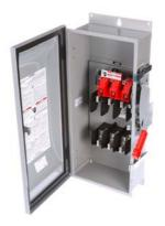
Siemens Low Voltage Circuit Protection Heavy Duty Safety Switches. Type: ENCLOSED, SAFETY SWITCH Std: CSA V. Rating: 240V A. Rating: 100A Wattage: 3W No. Of Poles: 3P F. Rating: 60Hz Action: SINGLE THROW Material: 304SS Enclosure: TYPE 12. 2-3 point mounting holes. Insulation: YES O. Cycles: 10000 O. Temperature: (-20F-120F) AMBIENT TEMPERATURE Environmental Conditions: INDUSTRIAL
