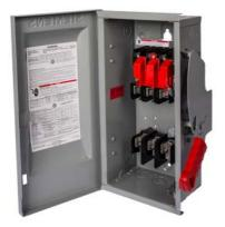
Siemens Low Voltage Circuit Protection Heavy Duty Safety Switches. Type: ENCLOSED, SAFETY SWITCH Std: CSA V. Rating: 600V A. Rating: 60A Wattage: 3W No. Of Poles: 3P F. Rating: 60Hz Action: SINGLE THROW Material: 304SS Enclosure: TYPE 3R. 2-3 point mounting holes. O. Cycles: 10000 O. Temperature: (-20F-120F) AMBIENT TEMPERATURE Environmental Conditions: OUTDOOR
