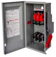
Siemens Low Voltage Circuit Protection Heavy Duty Safety Switches. Type: ENCLOSED, SAFETY SWITCH Std: CSA V. Rating: 600V A. Rating: 60A Wattage: 2W No. Of Poles: 2P F. Rating: 60Hz Action: SINGLE THROW Material: 304SS Enclosure: TYPE 3R. 2-3 point mounting holes. O. Cycles: 10000 O. Temperature: (-20F-120F) AMBIENT TEMPERATURE Environmental Conditions: OUTDOOR
