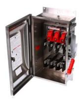
Siemens Low Voltage Circuit Protection Heavy Duty Safety Switches. Type: ENCLOSED, SAFETY SWITCH Std: UL V. Rating: 600V A. Rating: 60A Wattage: 3W No. Of Poles: 3P F. Rating: 60Hz Action: SINGLE THROW Material: SS Enclosure: TYPE 4X. 2-3 point mounting holes. Insulation: YES O. Cycles: 10000 O. Temperature: (-20F-120F) AMBIENT TEMPERATURE Environmental Conditions: INDUSTRIAL CORROSIVE RESISTANCE
