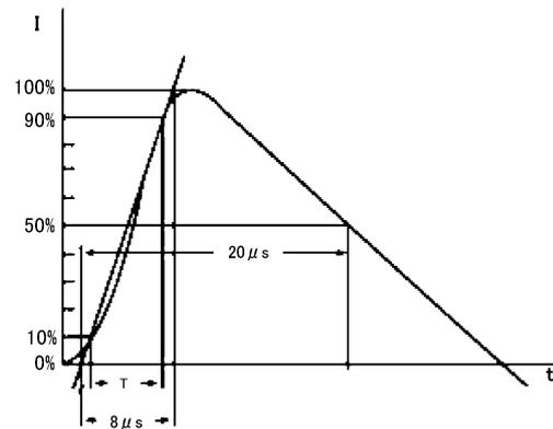
**Fig. 5.3.2 Based on IEC61000-4-5 8/20 μs pulse.**
