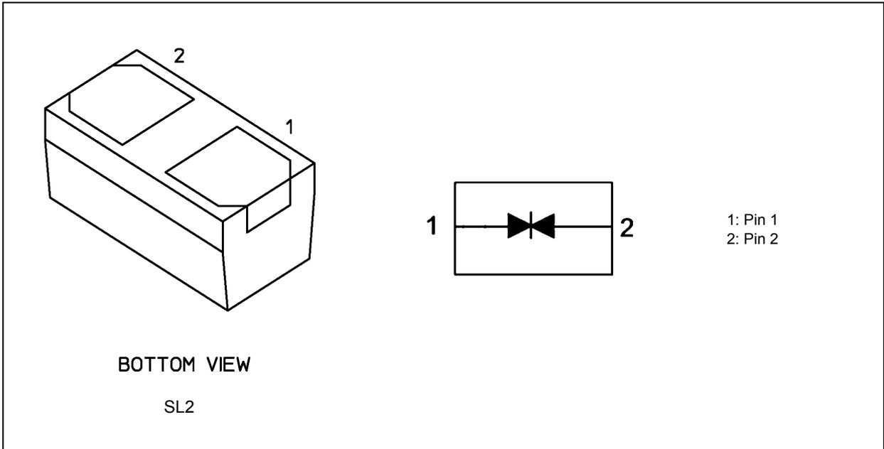
Note: Connect Pin 2 to GND when using Pin 1 for I/O.
