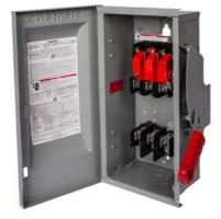
Siemens Low Voltage Circuit Protection Heavy Duty Safety Switches. Type: ENCLOSED, SAFETY SWITCH Std: CSA V. Rating: 240V A. Rating: 200A Wattage: 4W No. Of Poles: 3P F. Rating: 60Hz Action: SINGLE THROW Material: STEEL Enclosure: TYPE 1. 2-3 point mounting holes. O. Cycles: 8000 O. Temperature: (-20F-120F) AMBIENT TEMPERATURE Environmental Conditions: INDOOR
