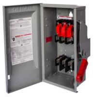
Siemens Low Voltage Circuit Protection Heavy Duty Safety Switches. Type: ENCLOSED, SAFETY SWITCH Std: CUL V. Rating: 600V A. Rating: 60A Wattage: 6W No. Of Poles: 6P F. Rating: 60Hz Action: SINGLE THROW Material: 304SS Enclosure: TYPE 3R/12. 2-3 point mounting holes. Insulation: YES O. Cycles: 10000 O. Temperature: (-20F-120F) AMBIENT TEMPERATURE Environmental Conditions: OUTDOOR/INDUSTRIAL
