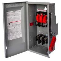
Siemens Low Voltage Circuit Protection Heavy Duty Safety Switches. Type: ENCLOSED, SAFETY SWITCH Std: CSA V. Rating: 600V A. Rating: 100A Wattage: 4W No. Of Poles: 3P F. Rating: 60Hz Action: SINGLE THROW Material: STEEL Enclosure: TYPE 1. 2-3 point mounting holes. O. Cycles: 10000 O. Temperature: (-20F-120F) AMBIENT TEMPERATURE Environmental Conditions: INDOOR
