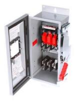
Siemens Low Voltage Circuit Protection Heavy Duty Safety Switches. Type: ENCLOSED, SAFETY SWITCH Std: UL V. Rating: 600V A. Rating: 30 A No. Of Poles: 3P F. Rating: 60Hz Action: SINGLE THROW Material: 304SS Enclosure: TYPE 12. 2-3 point mounting holes. Insulation: YES O. Cycles: 10000 O. Temperature: (-20F-120F) AMBIENT TEMPERATURE Environmental Conditions: INDLISTRIAL
