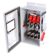
Siemens Low Voltage Circuit Protection Heavy Duty Safety Switches. Type: ENCLOSED, SAFETY SWITCH Std: UL V. Rating: 240V A. Rating: 100A No. Of Poles: 3P F. Rating: 60Hz Action: SINGLE THROW Material: 304SS Enclosure: TYPE 12. 2-3 point mounting holes. Insulation: YES O. Cycles: 10000 O. Temperature: (-20F-120F) AMBIENT TEMPERATURE Environmental Conditions: INDUSTRIAL
