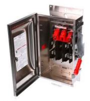
Siemens Low Voltage Circuit Protection Heavy Duty Safety Switches. Type: ENCLOSED, SAFETY SWITCH Std: UL V. Rating: 240V A. Rating: 60A Wattage: 2W No. Of Poles: 2P F. Rating: 60Hz Action: SINGLE THROW Material: SS Enclosure: TYPE 4X. 2-3 point mounting holes. Insulation: YES O. Cycles: 10000 O. Temperature: (-20F-120F) AMBIENT TEMPERATURE Environmental Conditions: INDUSTRIAL CORROSIVE RESISTANCE
