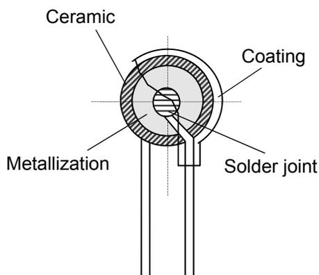
The above picture shows the internal construction of EPCOS ICLs.
