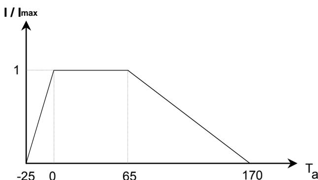
$$\text{Percent of } I_{max} = 100 \left[ 1 - \frac{T_A - 65^\circ C}{T_{max} - 65^\circ C} \right]$$
