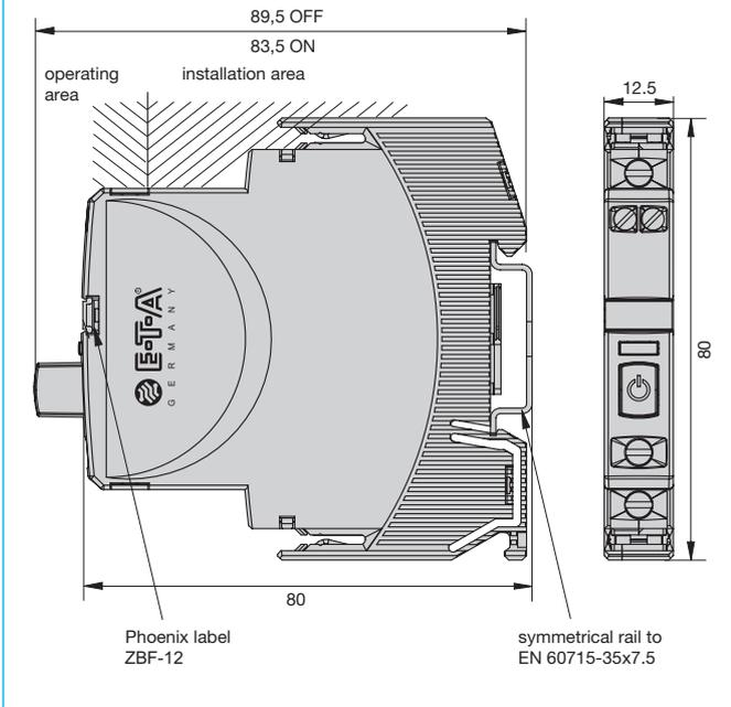
**Schematic diagram ESS31-T**
