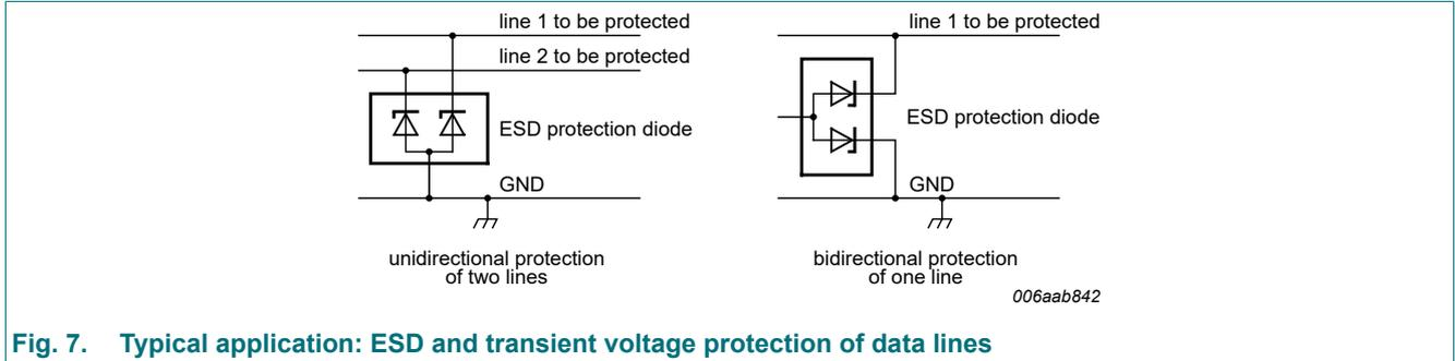
Fig. 7. Typical application: ESD and transient voltage protection of data lines
