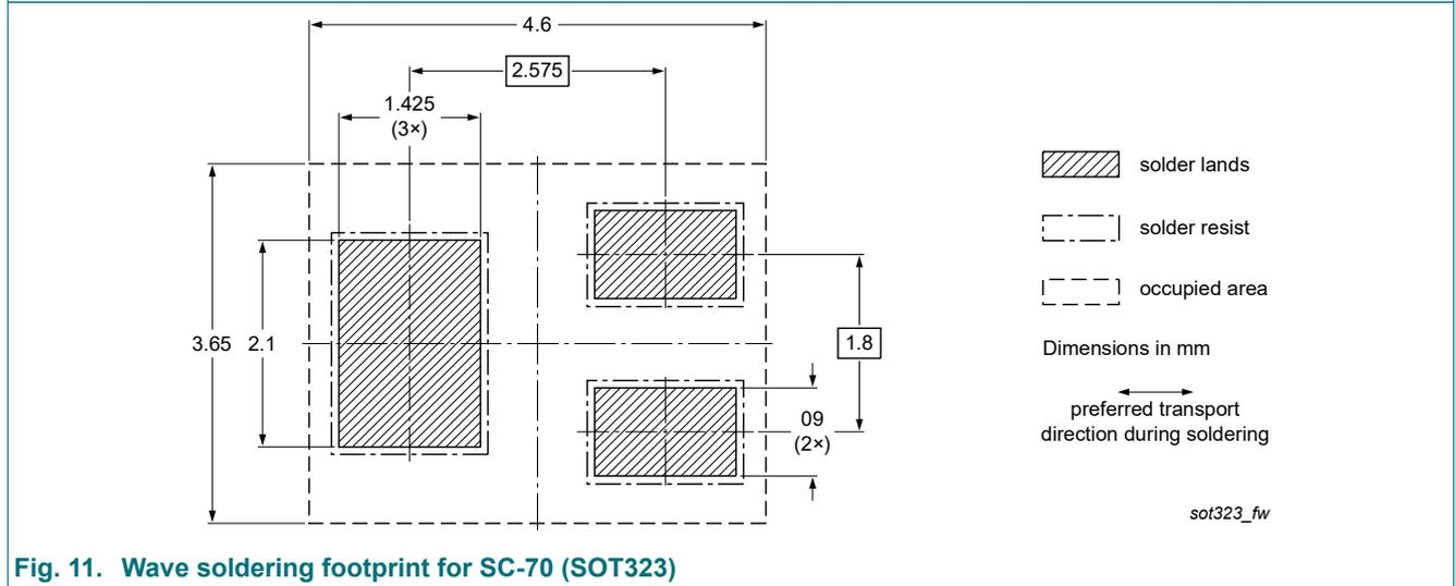
Fig. 11. Wave soldering footprint for SC-70 (SOT323)
