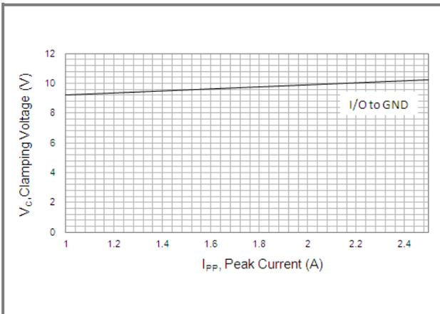
Fig.3 Typical Peak Clamping Voltage(8/20µs)
