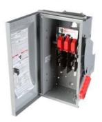
Siemens Low Voltage Circuit Protection Heavy Duty Safety Switches. Type: ENCLOSED, SAFETY SWITCH Std: CSA V. Rating: 240V A. Rating: 30 A Wattage: 3W No. Of Poles: 2P F. Rating: 60Hz Action: SINGLE THROW Material: 304SS Enclosure: TYPE 3R. 2-3 point mounting holes. O. Cycles: 10000 O. Temperature: (-20F-120F) AMBIENT TEMPERATURE Environmental Conditions: OUTDOOR
