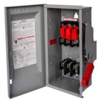
Siemens Low Voltage Circuit Protection Heavy Duty Safety Switches. Type: ENCLOSED, SAFETY SWITCH Std: CSA V. Rating: 240V A. Rating: 60A Wattage: 3W No. Of Poles: 2P F. Rating: 60Hz Action: SINGLE THROW Material: STEEL Enclosure: TYPE 1. 2-3 point mounting holes. O. Cycles: 10000 O. Temperature: (-20F-120F) AMBIENT TEMPERATURE Environmental Conditions: INDOOR
