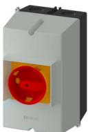
Cast aluminum surface mounting enclosure Degree of protection IP65 72 mm installation width, PE terminal with rotary operating mechanism yellow/red for circuit breaker Size S0
