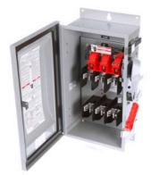
Siemens Low Voltage Circuit Protection Heavy Duty Safety Switches. Type: ENCLOSED, SAFETY SWITCH Std: UL V. Rating: 240V A. Rating: 60A Wattage: 3W No. Of Poles: 3P F. Rating: 60Hz Action: SINGLE THROW Material: 304SS Enclosure: TYPE 12. 2-3 point mounting holes. Insulation: YES O. Cycles: 10000 O. Temperature: (-20F-120F) AMBIENT TEMPERATURE Environmental Conditions: INDUSTRIAL
