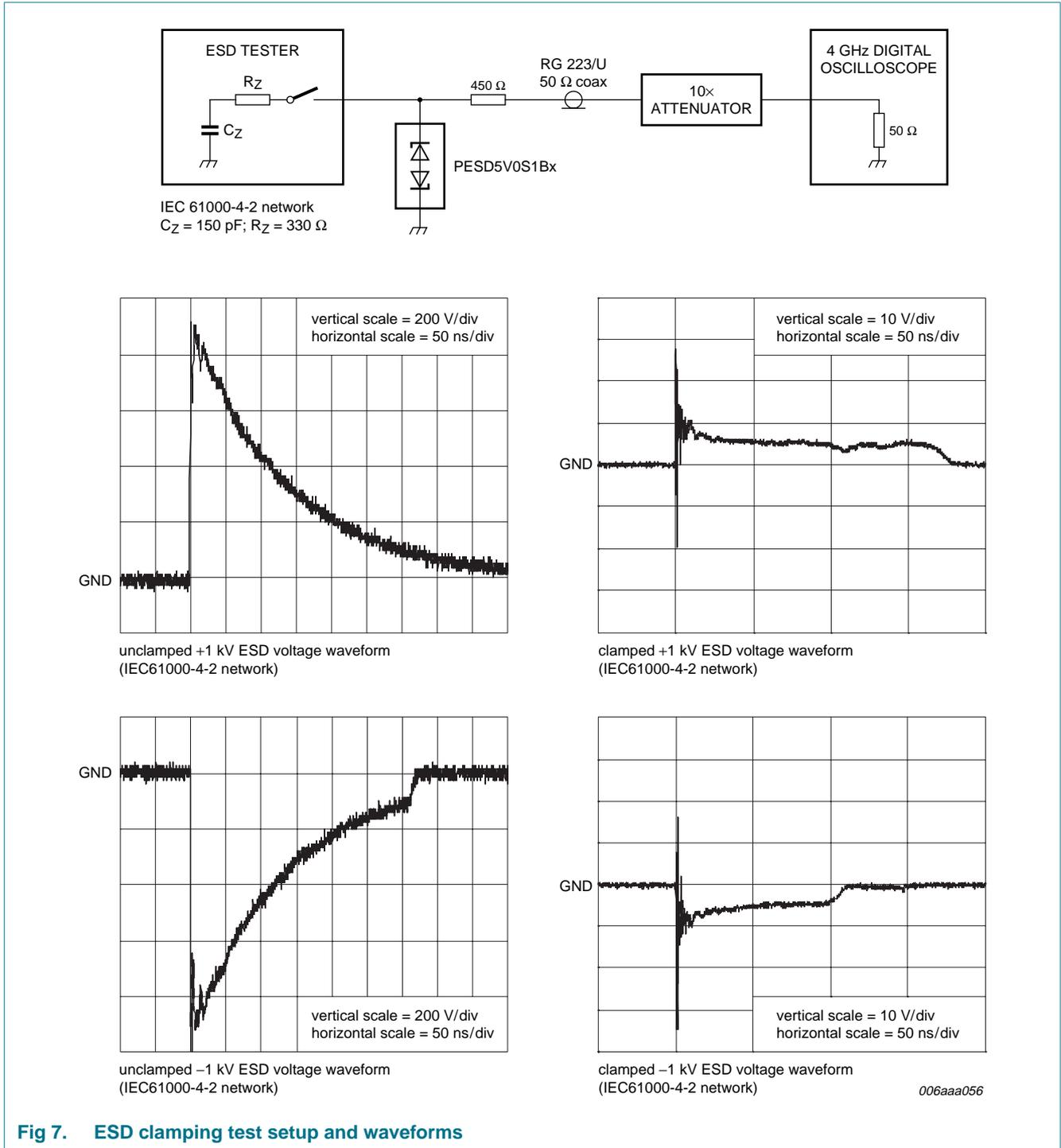
**Fig 7. ESD clamping test setup and waveforms**
