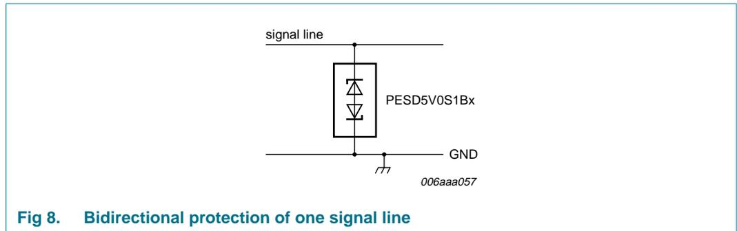
**Fig 8. Bidirectional protection of one signal line**
