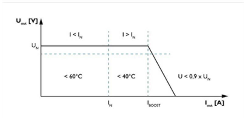
capacitive loads have to be absorbed without voltage dips. With this QUINT Power Boost function a static boost will continuously provide up to 125% of the nominal current.
