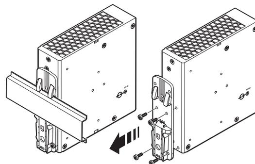
Figure 10 Disassembling the universal DIN rail adapter
