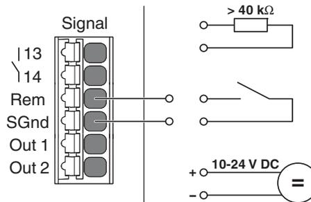
Figure 29 External wiring versions, disable SLEEP MODE
