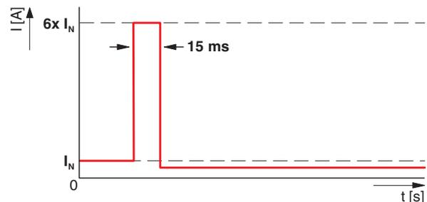
Figure 25 SFB pulse trips circuit breakers
