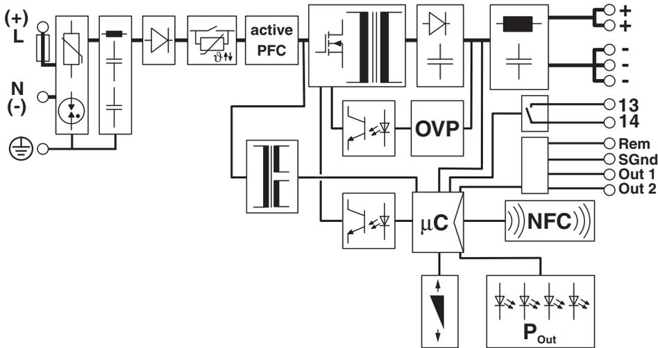
Figure 7 Block diagram
