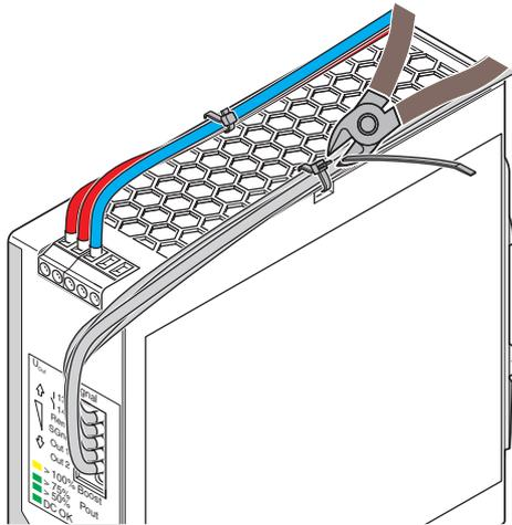
Figure 16 Shorten protruding ends of the cable binder
