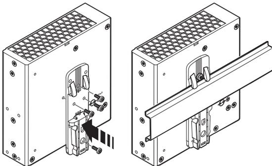
Figure 11 Mounting the universal DIN rail adapter
