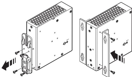
Figure 13 Mounting the UWA 130 universal wall adapter
