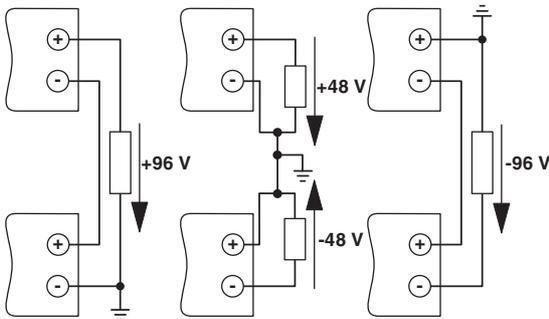
Figure 33 Schematic diagrams in series operation
