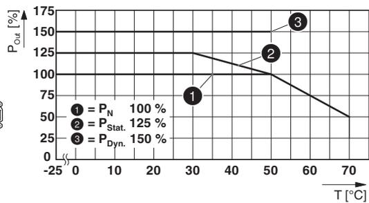
15.4.3 Rotated mounting position 180° X-axis
