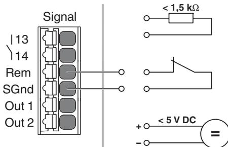
Figure 28 External wiring versions, enable SLEEP MODE
