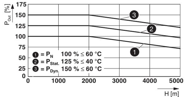
Figure 38 Output power depending on the installation height
