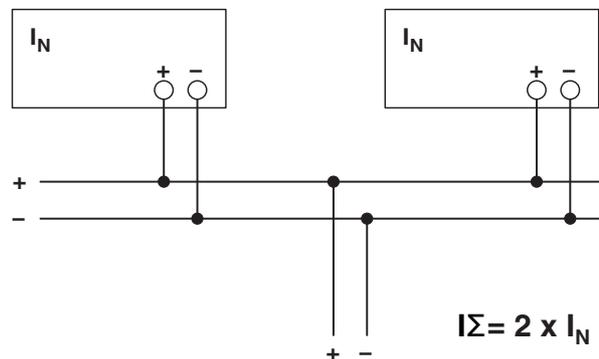
Figure 36 Schematic diagram of increased performance
