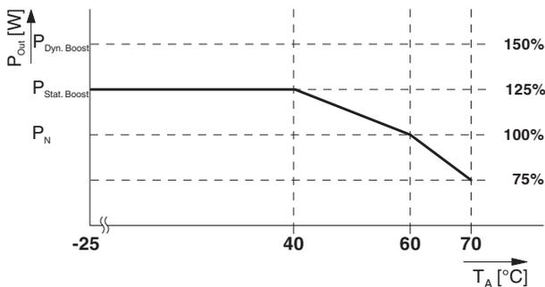
Figure 37 Output power depending on the ambient temperature
