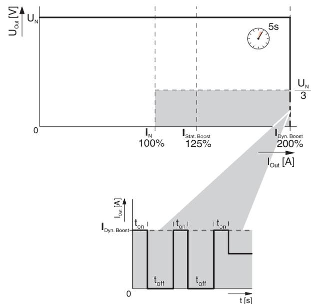
Figure 16 U/I Advanced output characteristic curve
