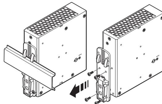
Figure 9 Disassembling the universal DIN rail adapter
