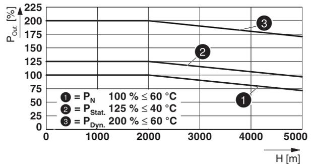
Figure 35 Output power depending on the installation height
