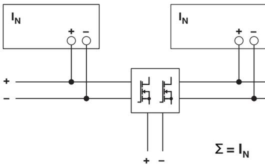
Figure 31 Schematic diagram, redundant operation with QUINT ORING
