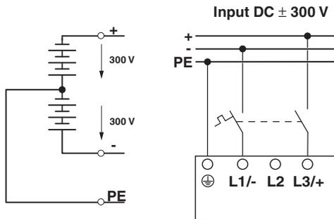
Figure 15 Pin assignment for DC supply voltage
