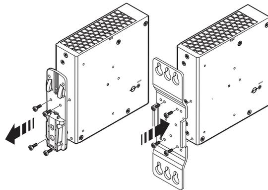
Figure 11 Mounting the UWA 182/52 universal wall adapter
