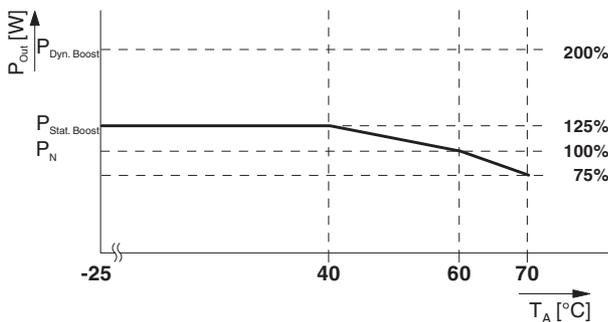
Figure 33 Output power depending on the ambient temperature
