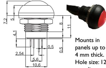
Mounts in panels up to 4 mm thick. Hole size: 12 mm dia.
