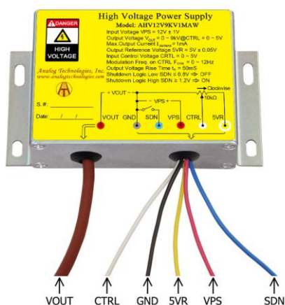
Figure 2. The Connecting Lead Wires of AHV12V9KV1MAW
