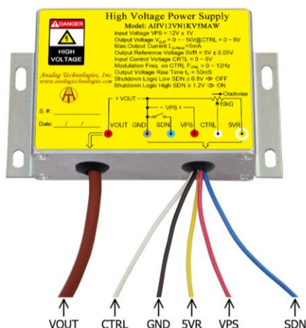
Figure 2. The Connecting Lead Wires of AHV12VN1KV5MAW
