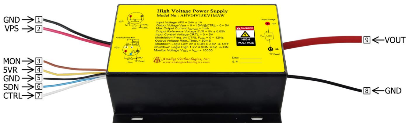
Figure 2. The Connecting Lead Wires of AHV24V15KV1MAW
